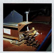
Rails rotated in virtually every application. In the upper photograph the rotation was initiated by the horizontal snubber pushing against the web of the beam. In both photographs the springs were secured by welding. Welding is always poor practice as the intense heat embrittles the spring so it tends to snap at the weld and scale inclusions produce welds that pop off. All systems failed with pipe breakage in addition to the other problems.
